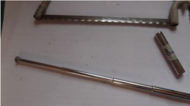
For holes of around 4mm to 8mm diameter - can you find an old telescopic antenna from somewhere? .... do you remember those they used to put on 35meg transmitters?
