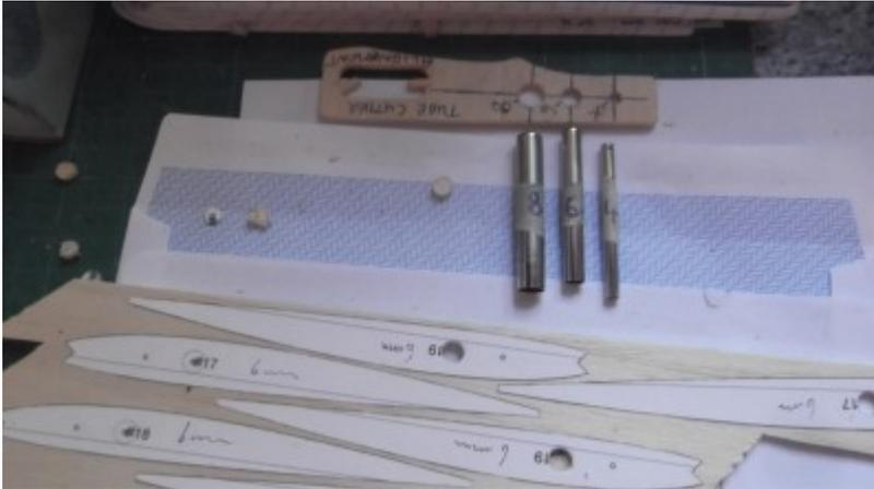
As you can see, what you do, is make a thin ply (about 2mm) alignment tool to fit a range of tube sized cutting tools.
