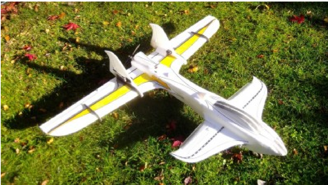
Early on the foreplane elevators were extended slightly with pieces of celluloid .... ... and now the rudders have like-wise been increased in area to give a more positive yaw control.
